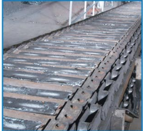
INGOT Casting Machine Conveyer
